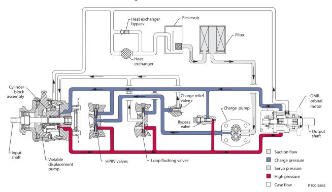
The diagram shows an LPV pump driving an OMR motor. The system shown uses an external charge pump and external filter. Charge pressure relief valves, high pressure relief valves, and loop flushing valves are shown separated from the pump to provide clarity to the hydraulic system.
