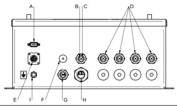
A Data output to operator terminals
