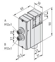
Casing, PA-GF, black Positive break Rated control supply voltage: 230 V AC Protection: IP 67, EN 60529 Test certification to BG-GS-ET-19
