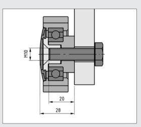
Rollers D60 PU can also be used as universal guide and support elements for pull-outs, as guide elements for sliding doors, and for all linear movements where flexibility and high load-bearing capacity are particularly important. They can be screwed from the outside (Countersunk Screw DIN 7981-M8) or inside (via the M10 internal thread) as required.
