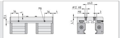
Machining requirements when using Slide Profiles LRF 8 in customised lengths. The indentations at the side offer a good point of orientation. The Slide Profiles allow users to locate mounting bores at will. The positioning collars can be used as necessary.
