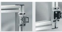
The actuator is available in two models – the fixed design is suitable for medium-sized sliding and swing doors (door width greater than 500 mm and smaller than 1000 mm), while the movable actuator is recommended for swing doors of width < 500 mm (angle compensation) and for particularly large doors.
