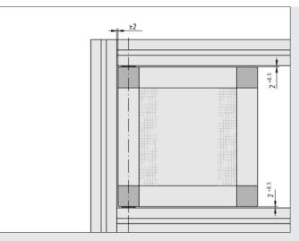
The Hinge Sets for installing swing doors in frame constructions of Line 5 or 8 contain all the parts required for one hinge.
