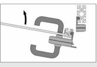
Swing door with inner-mounted lock, stop provided by the lock housing rabbet.
