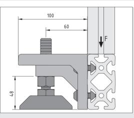
The maximum permissible load on the Foot Mounting Bracket is F = 4,000 N. The load-carrying capacity of the adjustable foot must not be exceeded.
