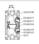
Installation example showing Installation Profile 8 160x80 K76 with the conduit divided using Partition Profile K76 K (0.0.663.47) and Partition Profile Clip K76 K (0.0.663.46). The maximum available clearance in the conduit is 30 mm in diameter.
