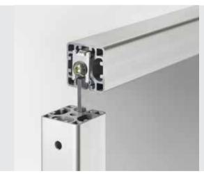
Standard-Fastening Set 8, one-sided has a modified centring feature that allows users to offset profiles. This means that right-angled profile connections can be achieved with a flush fit that factors in Caps (a). Furthermore, because the anti-torsion feature is located on just one side, the internal grooves are left clear. This means that panel elements can be inserted into the grooves without having to trim the corners first (b).
