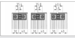
Possibilities for mounting the anti-torsion block with profiles
