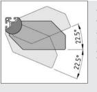
To allow the Light Fitting to be adjusted to individual applications, it can be locked in various positions over a swivel range of  $\pm 22.5^{\circ}$ from 0°.
