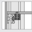
Profiles 8 40x32 and 80x32 light are particularly suitable for use as frames and struts in table, shelving and cabinet constructions. They are then used to connect profiles of modular dimension 40 mm.
