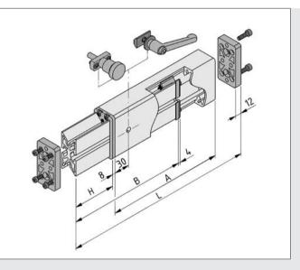
Telescope Inner Profile 8 80x40 (length B) must be 20 mm shorter than Telescope Profile 8 80x40 (length A) in order that it can be inserted completely in the assembled telescope, and stroke H thereby maximised.
