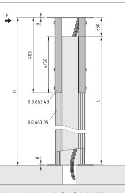
Maximum torsional moment for Base Plate, Installation Column Profile such as for cracked C20/C25 concrete and Floor-Fastening Set M10x135 (0.0.485.82):
