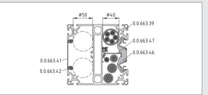
Installation example showing Installation Column Profile 8 160x160 K76 with the conduit divided using Partition Profile K76 K (0.0.663.47) and Partition Profile Clip K76 K (0.0.663.46). The maximum available clearance in the conduit is 40 mm in diameter. The maximum available clearance in the conduit when not using Partition Profile K76 K (0.0.663.47) and Partition Profile K76 K (0.0.663.46) is 50 mm in diameter.
