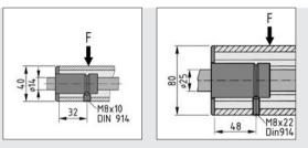
The Ball-Bearing Guide Bush Units are fixed in the cavities of Profiles 8 using grub screw DIN 914-M8.
