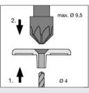
The machining required is limited to counter boring and countersinking of the Caps.
