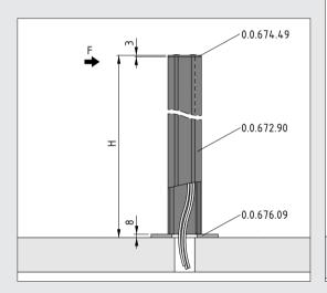
Maximum torsional moment for Base Plate, Installation Profile 160x80, such as for cracked C20/C25 concrete and Floor-Fastening Set M10x135 (0.0.485.82):
