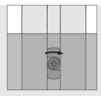
T-Slot Nut PA can, if required, be prefitted (using the screw) to the component to be secured and is inserted at any position in the profile groove.
