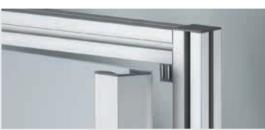
Magnetic Catches are particularly suitable for latching swing and sliding doors. Turning the Magnetic Catch through 180° enables users to choose between two different holding forces (this does not apply to Magnetic Catch X).
