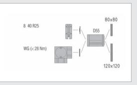
The connection dimensions and the permissible torque range ( $M_0 < 50$  Nm) make Coupling D55 ideally suited for use with Timing-Belt Reverse Unit 8 40 R25 with multi-spline VK14 (Centring Piece D50-D22) and (optionally) Bevel Gearboxes WG (Centring Piece D50-D50: note torque limit 28 Nm!).
