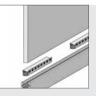
The number of Clamping Springs required depends on the load, the inherent stability and the size of the panel element.
