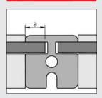
When planning panel element cut-outs, the penetration depth (a) specified here must be taken into account irrespective of the penetration depth specified for the Clamp Profiles.
