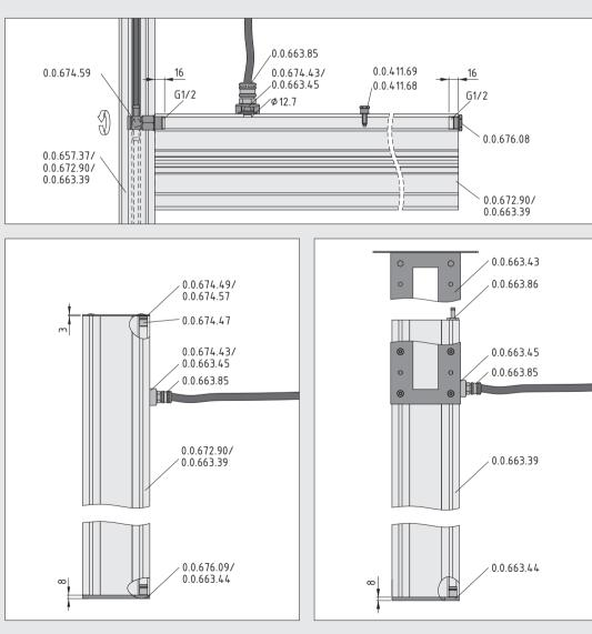
Example showing a horizontal Installation Profile fitted with various pneumatic components.
