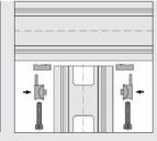
Fastening on the groove side is by means of a Pneumatic Universal-Fastening Set 8 or Automatic-Fastening Set 8.
