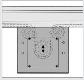
The Chain Counter-Reverse Unit is screwed directly to the Support Profile. The Chain Guide Profile must be interrupted at this point in order to remove the chain from the profile groove.
