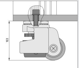
Jacking Castor D62 can be fitted directly to any Base Plate/ Transport Plate with an M12 and M16 thread using the enclosed Hexagon Socket Head Cap Screw and washer.
