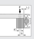
Recommendation for mounting the panel element. The permissible load for Multiblocks X 8 PA is F = 250 N.
