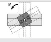
The angle between the profiles can be selected in  $5^{\circ}$  increments. The toothing ensures that the two halves fit together securely at the correct angle.
