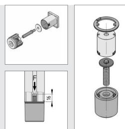
The spindle is screwed into an M8 thread in the core bore of the profile. Tools are not required to make height adjustments – simply turn the lower part of the foot manually.
