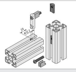
The pre-tensioning force of the Universal-Fastening Set (Profile St) 8 is applied by two screws which are tightened from the profile groove. They are screwed into T-Slot Nuts (Profile St) 8 M6, which are inserted in the opposite profile groove.
