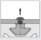
Tightening the screw automatically locks the T-Slot Nut in the groove.
