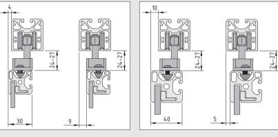
Runway Profile 8 40x40 with universal Profile 8 groove is easy to fasten and guides the sliding elements. The hanger has broad adjustment ranges for door frames made from Profiles 8.
