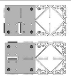
The Mounting Plate can be used to fasten Timing Belt R50 to any face of the profile.
