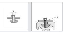
Required machining and fastening elements for fixing a Slide Guide Strip of any required length at the floating bearing end. The distance between the fastening elements should be
