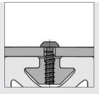
Button-Head Screw T4 from item has been specially designed for use with T-Slot Nut 8 PA. This screw cuts its own thread in the plastic body.
