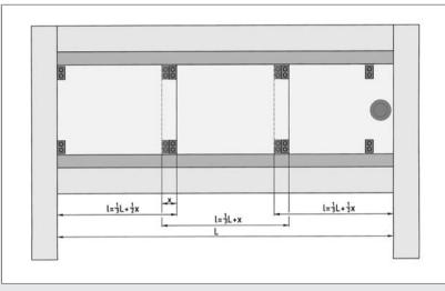
Typical arrangement of a 3-part sliding door with equal-sized door segments.
