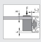
Recommendation for mounting the panel element. Permissible loading force for Multiblocks 8 is F = 250 N.
