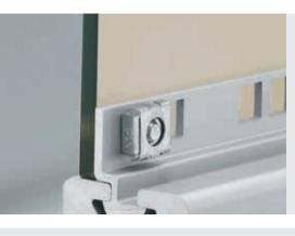
Universal usage for installation in Rebate Profile 8 Al 19" or in panel elements. The Captive Nuts can be installed by snapping the latch springs into the corresponding recess.
