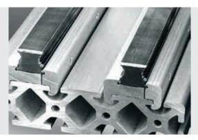
Profiled Linear Guide Rail with special rail base geometry. Clamping using the Guide Rail Mounting Profile and Guide Rail Clamping Profile makes it possible to use rails without holes that do not require Caps, or subsequent machining.
