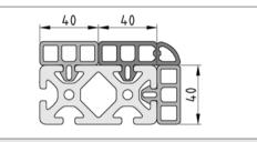
The Protective Profiles have a modular dimension of 40 mm.
