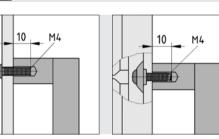
When using screws to fasten the Handle on profile grooves, it is advisable to use the appropriate Locating Washers.
