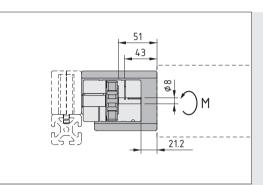
The Rack 8 Coupling Module fits nearly any motor – simply process the housing and coupling to suit your needs. You will, however, need to take care over how far the shaft extends into the coupling half.
