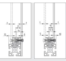
The length of the fastening screw depends on the thickness of the panel element.
