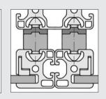
Attaching the Hanger from the front ensures that the frame and panel elements can be fitted without gaps.
