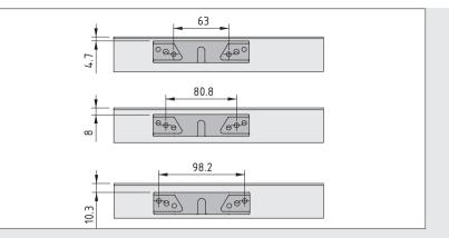
Processing of Profile M W  $40x25x2 \ \text{E}$  for maximum slide adjusting range
