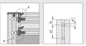
Position of the through holes for the key.
