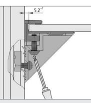
Support Arms X 6-8 are suitable for clamping panel elements 4 to 10 mm thick.
