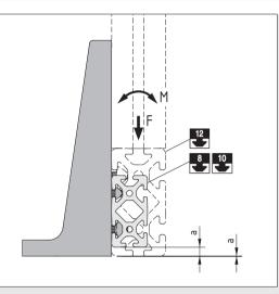
In the case of Line 8 profiles, the distance to the floor when using the lower groove for attaching the L-Based Foot is a = 9.5 mm. In the case of Line 10 profiles a = 4.5 mm. Line 12 profiles can be screwed to the L-Based Foot so that they are flush to the floor.
