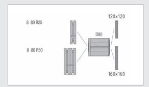
Coupling D80 is used with an appropriately sized Coupling Housing for the purpose of transferring the high torque ( $M_D < 100$  Nm) of Timing-Belt Reverse Units 8 80 R25 and 8 80 R50 II with multi-spline VK32. The Coupling Housing has a corresponding Centring Piece ( $\varnothing$  60 mm) for the Timing-Belt Reverse Units.
