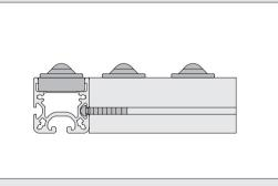
Interlinking two Castor Rails 8 40x40 using fastening elements and Profile 5 and 8 grooves.
