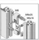
If the upper Hanger 8 is fitted to the Stand Profile and the lower Hanger 8 to the frame element, removal of Hexagon Socket Head Cap Screw M6 will result in the frame element being released.
