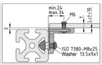
The panel element with through hole is secured by means of an M6 bolt fitted into the square nut of Multi Bracket 12 Zn.
