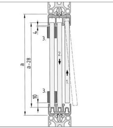
Use Clip 8 St to fasten the Sliding-Door Guide Profile to the frame profiles at the top and bottom. Next, insert the sliding doors as set out below:
