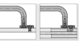
Handles AI can be secured from the rear (concealed). They can also be fitted from the front when used with the Fastening Sets.
