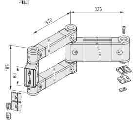
Double Pivot Arm 8 80 695 heavy-duty Profile 8 80x40 4N 180 E 2 Profiles 8 40x40 3N light End Swivel Joint 80 2 Double Swivel Joints 80 Connecting cover, PA, grey 3 Connecting Plates, Al, natural 3 Button-Head Screws M8x22, St, bright zinc-plated 3 T-Slot Nuts 8 St M8, bright zinc-plated Notes on Use and Installation  $F_{max.} = 250 \text{ N}$ m = 4.2 kg 1 set
