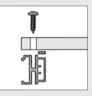
Sealing Strip, self-adhesive on one side, for sealing frame elements. Can also be used as a damping element on mating surfaces, particularly in combination with Double Panel Profile 8 Al.
