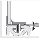
A screwdriver is used to lever out the Panel-Clamping Strip so as to enable removal of the panel element from the frame.
