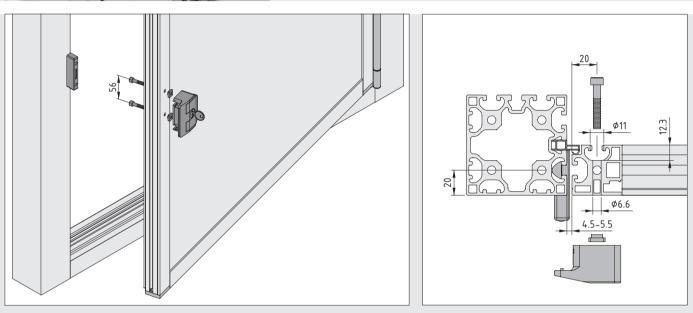
Door Lock X 8 Zn uses the profile groove in the door gap as a concealed fastening option. It can be installed at the ideal ergonomic height. All fastening screws are safely concealed when the door is closed.
