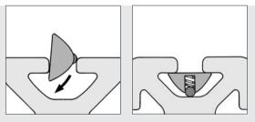
T-Slot Nuts St are inserted into the profile groove where they are secured in position by means of thrust pieces.
