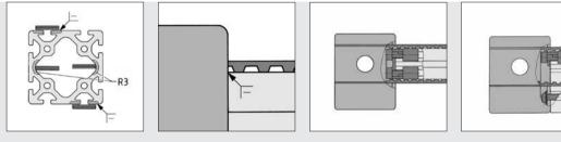
To protect the Timing Belt against damage, the profiles must be rounded at the joint to the Timing-Belt Reverse Unit. Timing-Belt Reverse Unit 8 40 R25 mounted at a height of 40 mm in the groove of Profile 8 using Universal Fastener 8 and special T-Slot Nut or in the core bore using Button-Head Screw ISO 7380-M8 and washer DIN 125-8.4. The special T-Slot Nut can be split in the centre and halved if required.
