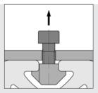
Tightening the screw automatically locks the T-Slot Nut in the groove. Pulling the screw fixes T-Slot Nuts 6 Zn and 8 Zn in the groove by means of the conical flanks.
