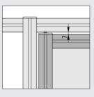
The gap between the door profile and the upper door frame must not exceed 7 mm.
