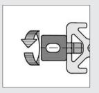
Twisting the Multiblock PA into the profile groove. The Multiblocks can be moved within the groove in order to align them with the bore in the panel element.
