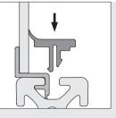
Panel-Clamping Strips consist of two components. The first of these, an aluminium strip, locates into the profile groove and holds the panel element in place. A second is then used to secure both the panel element and the If necessary, the plastic strip can be levered out in order to remove the panel element
