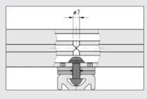
Two Line 8 Profiles are screw-connected using screw ISO 7380-M8x25, Washer DIN 125-8,4 and T-Slot Nut 8 St M8. An access hole must be made in one of the profiles to accommodate the Allen key.
