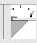
The permissible depth of the shelf is  $I_{max}$  = 200 mm with a load  $F_{max}$  = 80 N. The distance between two Support Arms should not exceed 500 mm.
