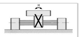
An individual Ball Bush is unable to absorb any moment. It is therefore always necessary to use two shafts for a guide system, with at least two Ball Bushes being located one after the other on a single shaft.
