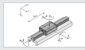
The permissible load for a linear guide system depends on the load bearing capacity of the guide elements but also on the strength of the screw connections and the construction of the profile frame.
