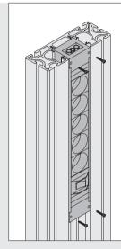
Distribution Strips and Multi-Socket Power Strips are fastened to the profile via screw connections.
