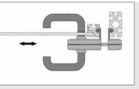
Lock System 6-8 fitted to a sliding door.
