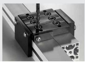
Because Drilling Jig 8 80, Standard Fastener 8 clamps to the outside of a profile, it can also be used on profiles with closed grooves. Suitable for Profiles 8 and Profiles X 8 up to a width of 80 mm.
