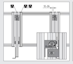
The captive security bolt: simply insert into the profile groove and tighten.
