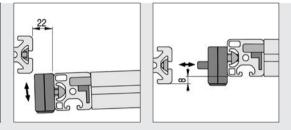
Application example for door construction: Clearance on left 28 mm with Hinges 8 40 Zn and on right 22 mm with Door Rabbets 8, in combination with Door Lock 8.
