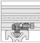
Installation note: Loosen the Cap Screw to maximise the adjustment range of the wedge and gently tighten the Countersunk Screw.
