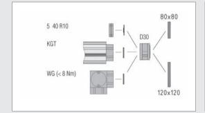
The connection dimensions and the permissible torque range ( $M_D < 8$  Nm) make Coupling D30 ideally suited for use with Ball Screw Units (Ball Screw Units KGT; Centring Piece D50-D50), Timing-Belt Reverse Unit 5 40 R10 with multi-spline VK14 (Centring Piece D50-D22) and (optionally) Bevel Gearboxes WG (Centring Piece D50-D50).
