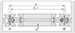
Slide Guide L (A = floating bearing) and Slide Guide F (B = fixed bearing) as guide elements, secured to a moving component.
