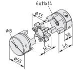
Coupling Half D55 D8, reborable up to  $\varnothing$  28 mm Coupling Half D55 VK14 Coupling Insert D55, hardness 98 Sh A Torque range: M<sub>D</sub> < 50 Nm Elasticity<sub>dyn</sub> = 0.009 °/ Nm Elasticity<sub>stat</sub> = 0.028 °/ Nm Perm. offset<sub>axial</sub> = 1.40 mm Perm. offset<sub>radial</sub> = 0.10 mm Perm. offset<sub>angular</sub> = 0.9 ° m = 280.0 g
