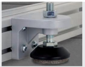
Foot Mounting Bracket 8 D80 allows height adjustable feet with M16 threaded spindle (primarily Knuckle Foot D80, M16) to be mounted on the side of a frame construction. Machines or systems can be installed with minimum distance to the floor but can still be adjusted in height.
