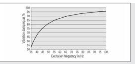
The effective height (h) when not under load is 9 mm. The value of h decreases by the spring distance a as a function of the force F. The degree of vibration damping depends on the excitation frequency. Shocks (excitation below the natural frequency) will be reduced by the self-damping.
