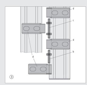
Various Hinge Leaves and Hinge Pins can be combined to
