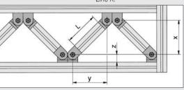
A Hinge heavy-duty can be fixed at any angle by pinning (a).
