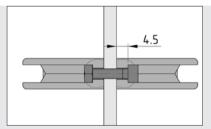
Handles PA for highly versatile application; they can be attached from the front or rear (concealed) and are particularly suitable for sliding and swing doors.
