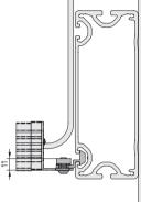
Because this robust, industrial quality Multi-Socket Power Strip can be fitted to the profile grooves of a machine frame or structure, positioning your power supply precisely where it is needed couldn't be simpler. Mains connection via a fixed conventional power cord that is included in the scope of supply. Multi-Socket Power Strip 19" is fitted to a Profile 8 groove using Rebate Profile 19".
