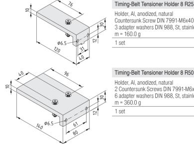
Holder, Al, anodized, natural Countersunk Screw DIN 7991-M6x40, St, bright zinc-plated 3 adapter washers DIN 988, St, stainless m = 160.0 g
