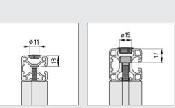
When screwing together profiles, users must drill through one profile to reach the core bore of the other profile. Cap 6 D11 and Cap 8 D15 seal this opening on profiles with closed grooves. This ensures that cut edges are safely covered over and keeps dust out of the grooves.
