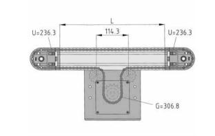
Calculating the chain length for a chain drive with two Chain Reverse Units 8 80 and one Chain Counter-Reverse Unit 8:
