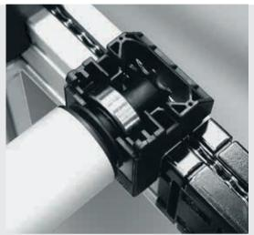
A simple ratchet mechanism is used to insert the Conveyor Rollers into the Bearing Blocks mounted on the frame profile.
