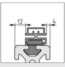
Matching to the wall thickness of the Panel Element by adjusting the positions of Double Panel Profile 8 Al and Clip 8 PA.
