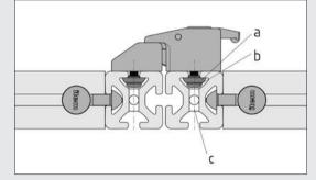
Door Lock 6-8 Zn screwed to profile door frame and fixed outer frame
