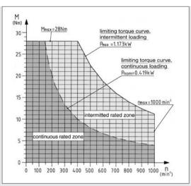
The diagram is used for calculating the permissible torques M and speeds n of the Bevel Gearboxes. For loads in the continuous rated zone, continuous operation is permissible. In the intermittent rated zone, operating times must be reduced accordingly.
