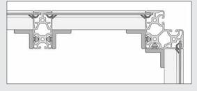
The Clamp Profiles light are connected using Angle Bracket V 8 40 Zn.
