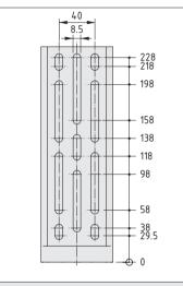
The slotted holes for fastening to the side face of a profile are compatible with the modular dimensions of Lines 8, 10 and 12.
