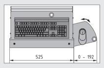
The mouse rest can be fitted to the right or left of the Keyboard Shelf.
