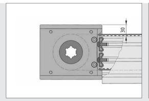
Connection of Timing-Belt Reverse Unit 8 80 R50 II based on a profile height of 120 mm (return of the Timing Belt in the profile cavity) or a profile height of 80 mm with Standard-Fastening Sets 8. To do this, the Timing-Belt Reverse Unit is partially dismantled, secured to the profile and then refitted.
