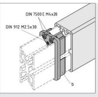
To secure the telescope cap (with Telescope Profile 8 80x40) and telescope sliding cap (with Telescope Inner Profile 8 80x40), the Telescope Connection Set is provided with self-tapping screws DIN 7500.
