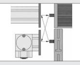
Attachment of drives (possibly with Adapter Flange Universal) and Timing-Belt Reverse Units to the Bevel Gearboxes with Adapter Plates. DIN931-M8
