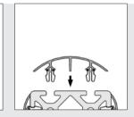
The round and flat Cover Profiles R, W and F are inserted into the grooves of Profiles 8 in conjunction with Clip 8 St.
