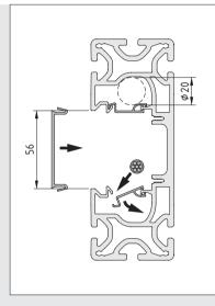
Cables measuring up to 20 mm in diameter can also be routed through Profile 8 160x60 4N K56 at any time after installation. Catch 40, Conduit Profile K retains cables in the internal conduits.
