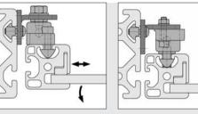
Application examples of a Catch Mounting Bracket with Ball Latch 8 for swing and sliding doors.
