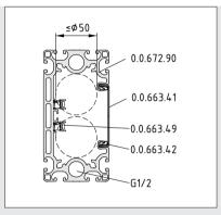
Installation example showing Installation Profile 8 160x80 K76 with Cover Profile 76 AI (0.0.663.41), Locking Clip St (0.0.663.42) and Earth Connection, Installation Column Profile (0.0.663.49). The maximum available clearance in the conduit is 50 mm in diameter.
