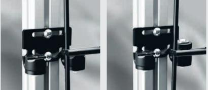
The Dual-Rod Mesh is first hung from a preassembled Dual-Rod Mesh Hanger, and then screwed into position with further Hangers. Recommended spacing of Hangers: 3 section heights, corresponding to 600 mm.
