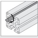
Profile Bars St are swivelled into the profile groove.
