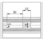
The openings are located at modular intervals and are used for running through cables and hoses. The Profiles are cut regardless of the positioning of the openings, therefore the minimum profile length is 160 mm.
