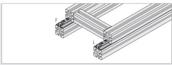
Slide guides with several slides must be designed as a combination of fixed bearing (F) and floating bearing (L). This compensates for tolerances and ensures ease of movement. The average coefficient of sliding friction of a T-Slot Slider is  $\mu = 0.22$ .
