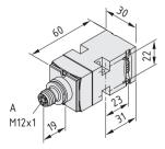
Casing, PA-GF, black Positive break Rated voltage: 24 V AC/DC / 230 V AC, 4A Protection: IP 67, EN 60529 Test certification to BG-GS-ET-15 Washers  $B_{10d}$  switch (NC) 2,000,000  $B_{10d}$  switch (NO) 1,000,000 Note: at 10% and with ohmic load Service life: 20 years m = 80.0 g 1 pce.
