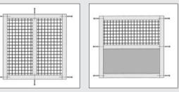
Where the panels are to be divided by a central strut (Clamp Profile 180°), this should always be tapped at the ends and bolted between the outer frame profiles.
