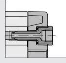
Supply of compressed air to a central bore by means of a Pneumatic Connecting Plate with Pneumatic Connection fitted to the end face.
