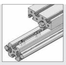
Arrangement of the plastic buffer in the groove of the supporting profile. Grub screw M8x44 is secured in the opposing groove of the moving carriage.
