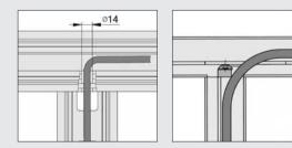
By providing Stand Profile 8 80x40 with a  $\varnothing$  14 mm bore, the profile can be used for routing cables and hoses.
