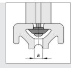
In addition, the Locating Washers allow Standard Con-nections (without anti-torsion element) between profiles of different Lines or they may be used simply to centre attachments.
