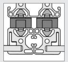
Attaching the Hanger from the front ensures that the frame and panel elements can be fitted without gaps.
