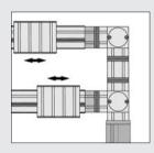
Parallel arrangement of Ball Screw Units in connection with Bevel Gearboxes.
