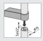
For longer Grip Systems X D25, an additional Hand Grip Element should be used to provide central support. Before being inserted in this Hand Grip Element, the second Profile D25 must be countersunk around the core bore.
