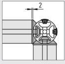
The gap that would result when connecting the rounded outer surface of Profiles 8 D40 and the straight profile end faces (or any other flat components) is closed off completely by Adapter 8 D40. A smooth transition is made from the outer contour of the profile to the connecting face of the second profile.
