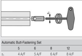
The Fastener is screwed into a profile groove in the end face, the thread being cut automatically. Use of a lubricant is recommended.
