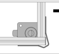
Installation examples showing Corner Deflector Guard 8 St 160x160x80 on basic constructions made of Line 8 profiles:
