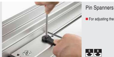
For adjusting the eccentrics on roller guides and C-Rail Guides
