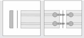
Seals PE must be used between all joints.
