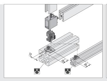
The hinge inserts are also fitted into the corner fasteners after the clamp profile frame has been closed.
