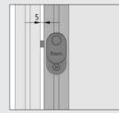
The gap between the door profile and the lateral door frame must not exceed 5 mm.
