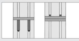
Possibilities for butt fastenings with Adapter Plates and Automatic Fasteners.
