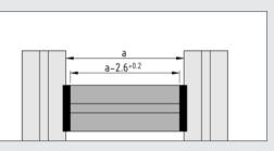
In calculating the length of the cross profiles between two profiles, the thickness of the Radius Seals on each side must be taken into account.
