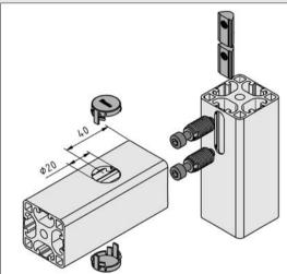
The fastener is located inside the profile cavity. To access the fastening screw just drill a hole into the profile. The grey Cap is used to close the hole.
