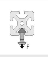
Permissible tensile load F on the groove flanks. This nominal load incorporates safety factors (S > 2) that act against deformation and fracturing. F = 750 N
