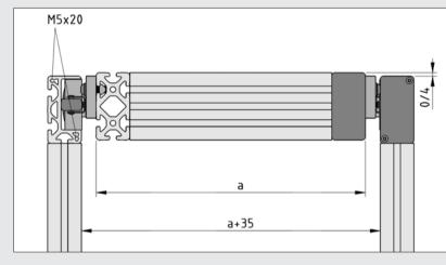
Track Profiles and Roller Units are also ideal for constructing overhead suspension units. An additional guide roller on the base plate guides Roller Unit D60 PU laterally in the Track Profile.
