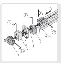
The basic components for an adjustment device include the Positioning Set 8 40 (1), the associated Feed Screw M6-LH (2) and the Handwheel D50 (3).
