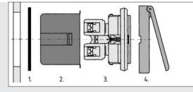
Sequence for installing Flush-Mounted Socket with lid:
