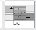
There can be either 1 or 2 sliding doors in a single Profile 8 groove.
