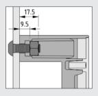
An M8 nut can be inserted in the lower part of the grip for fastening from the back of the door.
