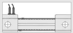
Possible arrangement of Proximity Switches 8 and Proximity-Switch Cams 8:
