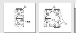
To protect the Timing Belt against damage, the profiles must be rounded at the joint to the Timing-Belt Reverse Unit.
