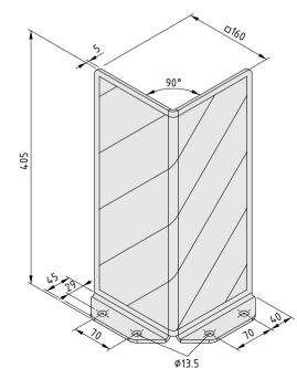
Collision Guard L With Hazard Markings
