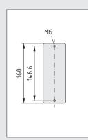
The M6 threaded bores in the mounting plates can be used in combination with Automatic-Fastening Sets 8 to connect the columns to Profiles 8 160x60 4N E.
