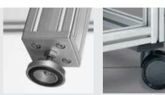
The Base Plates/Transport Plates, made from die-cast zinc, are powder-coated on all sides and can be screwed into the core bores of profile end faces or laterally into the grooves of the profiles.
