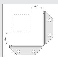
A clearance of at least 60 mm must be maintained to ensure compliance with the DGUV regulations.
