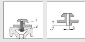
Required machining and fastening elements for fixing the Slide Guide Strip at the fixed bearing end.
