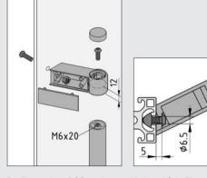
Profile sections D25 are inserted in Hand Grip Element X D25 from one or both sides. Any hole not required is covered using the Cap provided.
