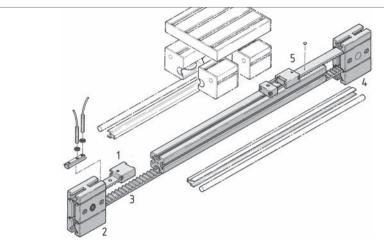
Timing-belt drives are particularly suitable for high speeds and extended stroke lengths.
