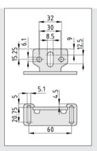
The connection is made on the profile side using M5 screws fitted into slots. DIN 125 washers must be used.
