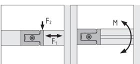
Where there is a combination of radial ( $F_1$ ) and axial ( $F_2$ ) load, the total load must satisfy the following equation:
