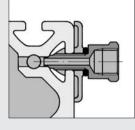
Supply of compressed air to the profile cavity by means of a central bore in the T-slot in conjunction with a Pneumatic Connecting Set. The seal is provided at the taper seat of the Pneumatic Connector.
