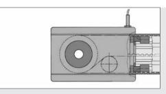
The variation in the emergence dimensions from 80 mm to 40 mm is achieved by rerouting the Timing Belt internally. The Timing Belt is routed with its smooth reverse side over the reversing pulleys.
