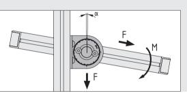
An adjustable profile frame with 2 Angle Locking Brackets 8 80x40 can withstand a force  $F_{max}$  = 2000 N. This profile frame has a permissible loading moment of: M = 100 Nm
