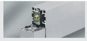
Standard-Fastening Set ESD is used in the same way as a conventional Standard-Fastening Set. The special design of the fastening screw partially destroys the insulating anodized layer on the profile groove and creates an electrical contact between the connected profiles.
