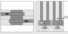
There can be either 1 or 2 sliding doors in a single Profile 8 groove.
