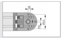
The Chain can be driven directly using the Chain Reverse Units or the Chain Counter-Reverse Unit. The sprocket wheels of the Chain Reverse Units are available with multispline hub VK14 or with a bore that can be machined as required. Use of multi-spline hub VK14 enables the modular accessories (Synchroniser Shafts) to be used without any restrictions.
