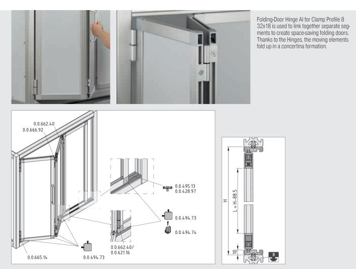
The sections of a folding door can be fitted with Rollers for Corner-Fastener 8 32x18 (0.0.494.74), as shown above. They run in Sliding-Door Guide Profile 8 40x10 (0.0.495.13), which must be taken into account when calculating the height of the door frame.
