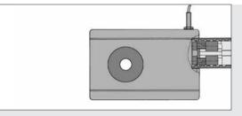
Timing-Belt Reverse Unit 8 80 R25 mounted at a profile height of 40 mm in the groove of Profile 8 using Universal Fastener 8 and special T-Slot Nut or at a profile height of 80 mm by splitting the special T-Slot Nut at the specified break point.
