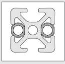
Automatic-Fastening Set 5 should be inserted so that the flattening on the thread is flush with the outer edge of the profile.
