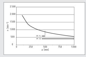
The permissible speed of a Synchroniser Shaft depends on its length.
