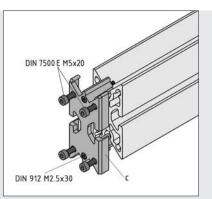
After assembly of the two telescope profiles, the plain bearings of the Telescope Sliding Cap and Telescope Cap are adjusted free of play using screws M2.5x30 (1.5 A/F).
