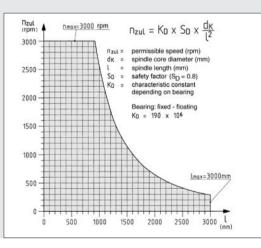
The Ball Screw Unit KGT can be driven from the fixed or floating bearing end.
