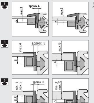
Two mounting dimensions are available depending on the orientation of the Multiblock.
