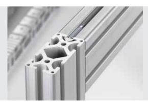
The Automatic-Fastening Set is an innovative solution for power-lock connections between profiles. Because no profile machining is required, it can be fitted quickly and easily. Due to the special design of the fasteners in the set, screw connections are all that is needed to fix them in place. They can be retrofitted to structures and repositioned in a matter of moments.
