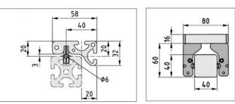
Basic construction of Profiles 8 with Roller Guide 8 on Shaft D6.
