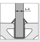
N.B.: Double-Lip Seal 8 is best installed using soapy water. It is then slipped onto the panel element and pushed into the profile groove. The profile frame is assembled around the panel element.
