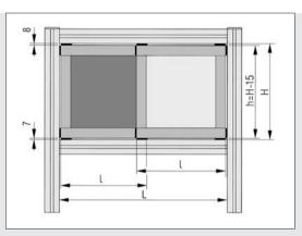
For sliding door constructions with n door elements of the same size, the following equation can be used to calculate the profile length I:
