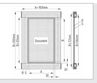
Calculating the number and lengths of the individual components for constructing Document Holders in the form of a clipboard.
