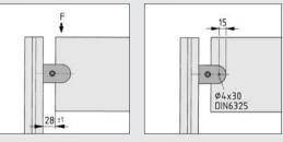
Max. loading for each Panel Clamp without pinning.  $F_{max} = 100 \text{ N}$
