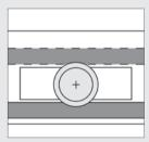
C-Rail System 1R with slides on prismatic steel rollers mounted on ball bearings and a polished guiding shaft. A second guiding shaft can also be fitted in order to prevent the sliding door from tilting when moved.
