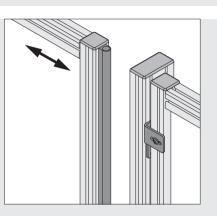
In enclosure and guard applications using Hanger 8/Door Rabbet 8 (gap width 25/28 mm), Buffer Strip 8 20x18 can be used to reduce the gap width.
