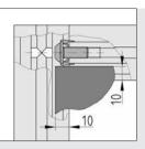
We recommend that panel elements be inserted to a depth of 10 mm into a Profile 8 groove.
