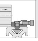
Direct-Fastening Set 8  $M_{stainl.} = 4.5 \text{ Nm} \text{ m} = 37.0 \text{ g}$
