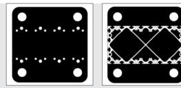
Base Plate 8 320x320 St has been prepared for screwing into the core bores of the profiles (8 countersinks for Hexagon Socket Head Cap Screws DIN 7984-M12 in Profiles 8 320x160 and 8 160x160, and countersinks for Hexagon Socket Head Cap Screws DIN 912-M8 in Profiles 8 160x160 8EN or 8 240x160 8EN).
