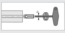
The Fastener is screwed into a profile groove in the end face, the thread being cut automatically. Use of a lubricant is recommended.
