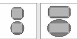
To achieve a completely smooth surface, both the Cap of the rectangular base profile and Caps R or F for the segments of the relevant Cover Profile must be used.
