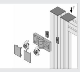
Fastening Hinge X 8 Zn to Line X 8 Profiles. For Profiles with closed grooves, the groove cover is to be removed to insert the T-Slot Nuts and positioning guides.
