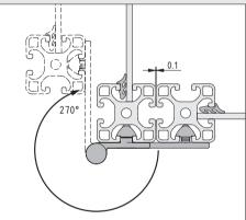
Hinges Al FP0-270° feature hinge leaves in different lengths. This enables an opening angle of 270°. The surface-mounted hinges secure both frameless panels and profile frames containing panel elements. Thanks to precision guidance that prevents the door leaf from sinking down, doors can be easily installed with virtually no gap between door and frame.
