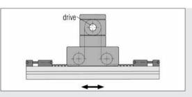
When fastening and tensioning the Timing Belt on a sliding carriage or support profile (using Counter-Reverse Unit 8) a Tensioning Block is required for each end of the Timing Belt.
