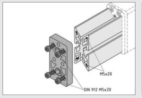
Telescope Connecting Plate 8 80x40 offers various possibilities for attaching the inside profile to a connecting structure. It is used for screw connection with Line 8 components or other parts. Suitable through holes and countersinks are provided in the Connecting Plate for this purpose.
