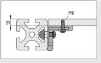
If the panel element is of sufficient thickness, Multi Bracket 12 can also be secured internally so that the fastening is not visible and cannot be detached.
