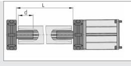
Use of a synchronising shaft for connecting two Timing-Belt Reverse Units.
