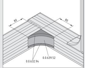
Conduit Inside Corner, Wall on modular conduits, wall height 80 mm: The wall profiles are each shortened by 80 mm. Using the Conduit Inside Corner, Lid:
