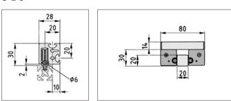
Basic construction of Profiles 5 with Roller Guide 5 on Shaft D6.
