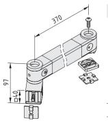
Profile 8 40x40 3N light End Swivel Joint Standard Swivel Joint Connecting cover, PA, grey 2 Connecting Plates, AI, natural Button-Head Screw M8x22, St, bright zinc-plated Notes on Use and Installation  $F_{max}$  = 120 N m = 1.4 kg 1 pce.
