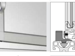
с. С Making sure doors keep themselves shut: The Magnetic Door Stop for Clamp Profile 8 32x18 is the ideal complement to Clamp Profile 8 32x18 (0.0.373.67), which can be used to build windows and doors with especially narrow frames. Clamping springs in a special groove on the Clamp Profile hold the panel elements steady and firmly in place.
