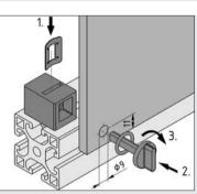
Quick Multiblocks can be used for panel elements of any thickness (up to 8 mm). They can be adapted to the thickness of the panel thanks to two different mounting positions (4 or 8 mm from the edge of the profile). The spring clip is to be inserted in the Quick Multiblock according to the direction in which the load is applied.
