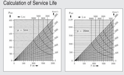
The service life of the spindle / drive nut combination can be calculated as a function of the axial load and drive speed.
