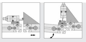
Fastening Set 6-8 is suitable for universal fastening of the Security Limit Switch/Security Lock compact and the actuator to Profiles 6 and/or 8. The slots allow customised adaptation to the direction of actuation and the position of the elements in relation to each other.
