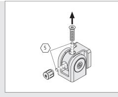
The Ball-Bearing Hinge can be screwed to any components using the integrated M8x16 fastening screws. These screws are driven through the holes in the bearing block using a 5 A/F hexagon key. To access the screws, simply remove the retaining screw from the bearing block. The Ball-Bearing Hinge does not need to be disassembled.
