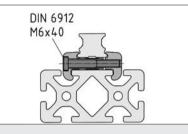
Linear Guide Rail PS 4-25 uses fastening profiles to create a clamping effect. A Guide Rail Mounting Profile, a Guide Rail Clamping Profile and the appropriate number of Hexagon Socket Head Cap Screws DIN 6912-M6x40 are required to mount each guide rail. The screws connect the two components of the linear guide system while the fastening profiles do not need to be machined.
