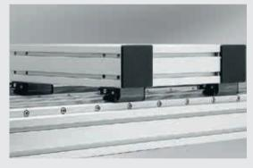
Guide systems with parallel rails on a single supporting profile can be constructed on the profile groove without elaborate alignment measures due to the special fastening geometry employed by the rail. The use of parallel rails on independent profiles or different support constructions will require the amount of alignment and fastening which is typical for profile rail guides (machining of location surfaces, use of parallel segments etc.).
