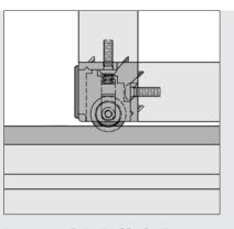
Spring-loaded Roller Set 32x18 is fitted into the corner fasteners of the previously constructed clamp profile frames. A Roller Set must be installed in each fastener so as to guide the sliding door leaf.
