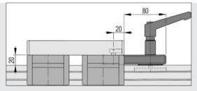
The special design of Slide Clamp 8 heavy-duty prevents undue force being applied to the bearings as a result of the clamping action.
