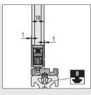
Sliding-Door Guide Profile 8 40x10 is fitted with Clip 8 St at the top and bottom of the surrounding profile frame. It forms the guide for two door leaves of Clamp Profile 8 32x18.
