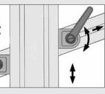
Combination of two Angle Clamp Brackets, e.g. for adjusting a rest (in terms of height, lateral location and angle).
