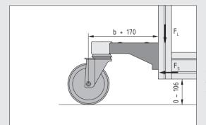
Castor Support 8 80x40 ensures that your construction has a low centre of gravity.
