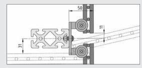
Average dimensions for connecting the Dual-Rod Mesh to the Stand Profile.
