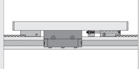
Universal connection bores in the carriage plate: M8 threaded holes for fastening profiles or any other structures. The driving force:
