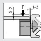
Recommendation for mounting the panel element and permissible loading forces for Multiblocks PA.
