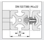
Special T-Slot Nut 8 Zn M4e with a central offset of 1 mm is available for moving elements made of Line 8 components. This ensures no collisions can occur during movement.
