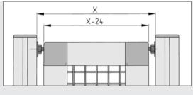
The clearance dimension between frame and Stand Profile is 12 mm. Dimensional tolerances of  $\pm$  3 mm can be accommodated by the Clamp-Profile Hanger E.
