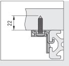
The table top does not need to be processed. The self-tapping screw can be screwed directly into the table top using a screwdriver (TX30 bit). The tolerance is adjusted by means of a slot in Table-Top Fastening Set 8.
