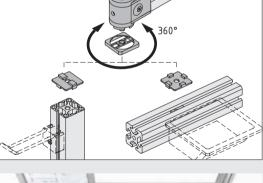
The connection can be made with either a horizontal or vertical profile groove. An end-face connection with Profiles is also possible. All the joints can be rotated through 360° and their frictional moment can be adjusted.
