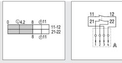
Illustration of circuits: Security Limit Switch compact 2NC Wiring diagram: Security Limit Switch compact 2NC
