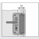
The door gap does not depend on the profile line used.
