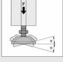
A ball and socket joint compensates for slopes.
