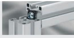
Standard-Fastening Set 8 K is a special version of the proven Standard-Fastening Set. It is employed for right-angled connection of Line 8 Profiles in which the profile grooves are used for holding panel elements.
