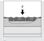
The maximum permissible load on a Chain Transfer Unit is calculated from the number of supporting links. For each chain link,  $F_{max} = 6$  N. Note the chain's operating load!
