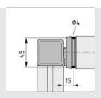
The circumferential groove in the bearing flanges also enable the Conveyor Rollers to be driven by a round belt  $\varnothing$  4 mm, if desired.
