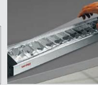
The Light Fitting can be sealed against dust (IP 40) by means of the Protective Panel. This panel also protects the Light Fitting against soiling and damage. The open socket must be sealed with a cap.
