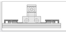
Drawing of a linear drive with moving axis. Holders prevent the timing-belt tensioners lifting away from the profile.
