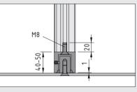
Partition Adapter D40 allows users to adjust the height and angle of each individual partition segment.
