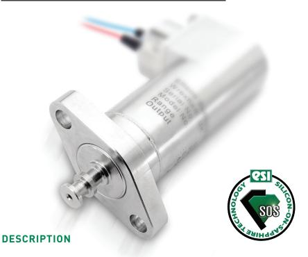
The PR3913 Valve-Mountable pressure transmitter has been designed to meet the requirements of the sub-sea oil industry and is configured to mount directly to the industry standard control valve flange arrangement.
