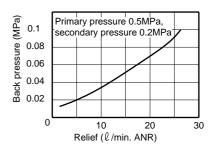
Note 1: With common exhaust, primary pressure is insufficient when using multiple manifolds simultaneously. So, install air supply block per three stations. Use an air supply port larger than OUT port size.
