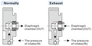
Normally, as the pressure of intake (IN) is higher than the set valve(pressure of outlet), the reverse flow valve closed; if the pressure of intake(IN) is cut off and starts exhaust, reverse flow valve opens. The pressure of diaphragm chamber is exhausted from IN orifice. At this moment, the pressure of diaphragm chamber decreases and the diaphragm is pressed down by the force from adjusting spring to open valve. The pressure from outlet is exhausted from IN port.
